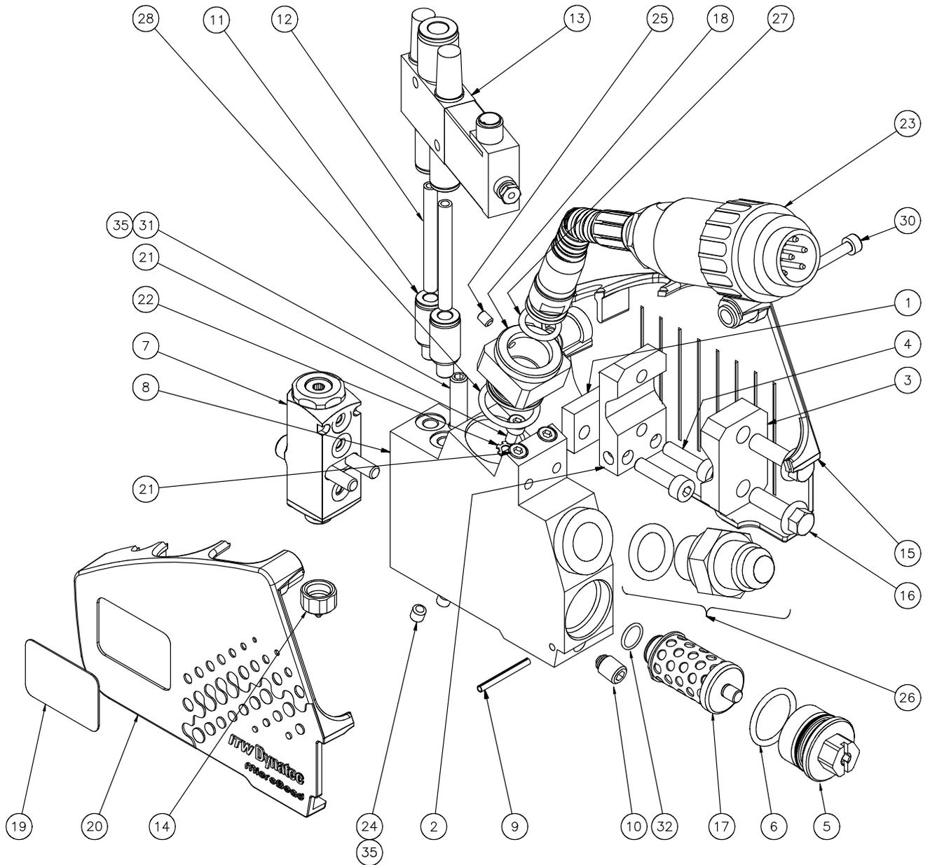
Component Illustration for BF MicroBead Applicator with One Module
