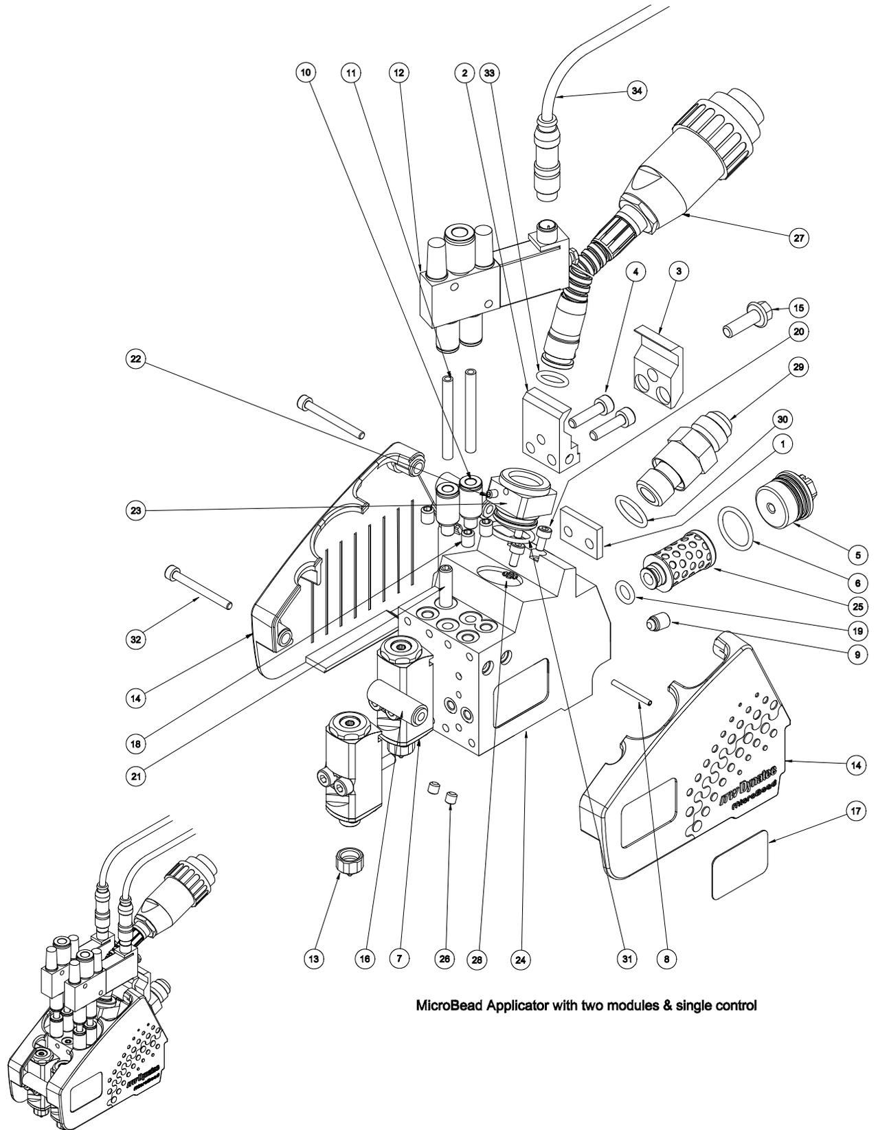
MicroBead Applicator with two modules & single control
