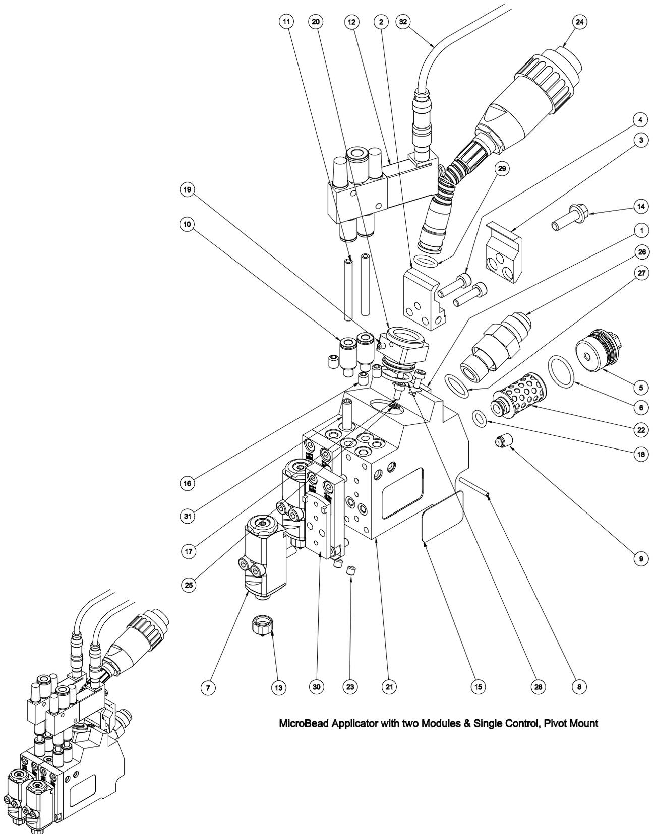
MicroBead Applicator with two Modules & Single Control, Pivot Mount
