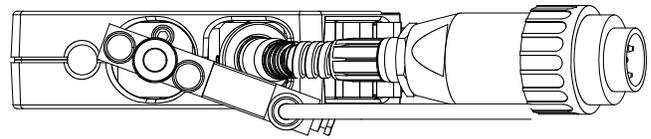
Upper view - Applicator and Micro Optima Module with integrated nozzle
