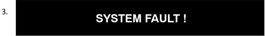
This fault, seen on the controller display, will result if the V6 modules on the DIN rail are not connected properly. A bus connector, near the rail, connects one module to the next. Modules can become disconnected during transport or during repair procedures.
